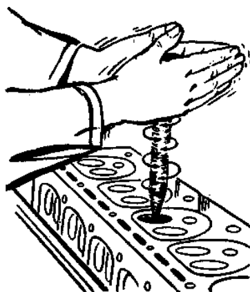
Lapping the valve and seat by hand—typical
