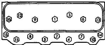
Big block V8 cylinder head bolt tightening sequence
