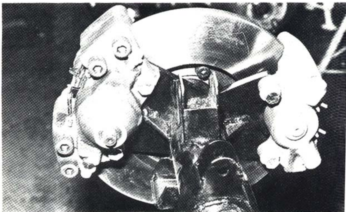
Above: Complete rear hub assembly. Below: Axle tube, spring saddle, bumper mount, top link mount and calipers on completed rear axle.
