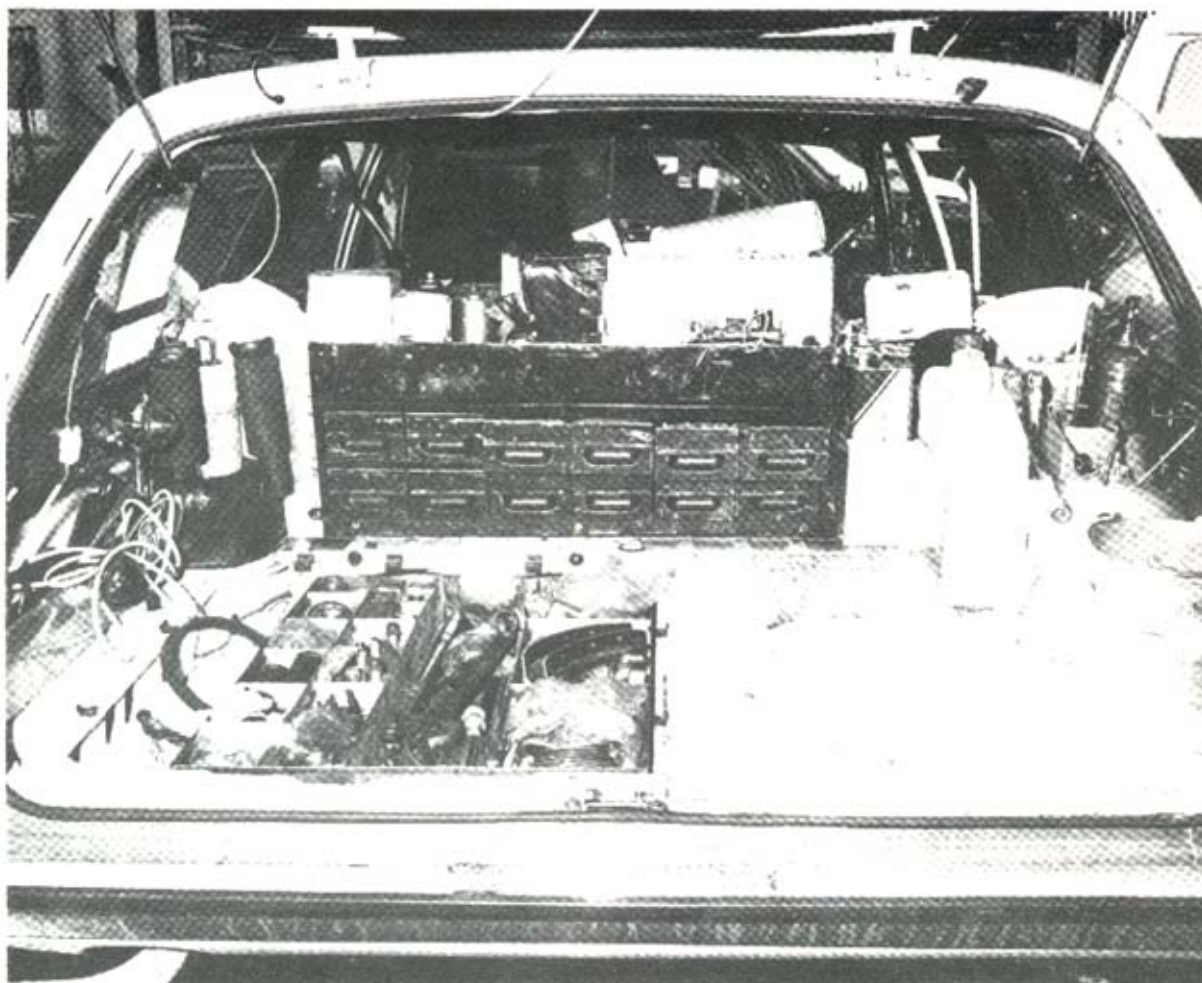
Back of Granada Service car. Spare wheel recess is used for quick access parts. Wheel goes on the roof.
