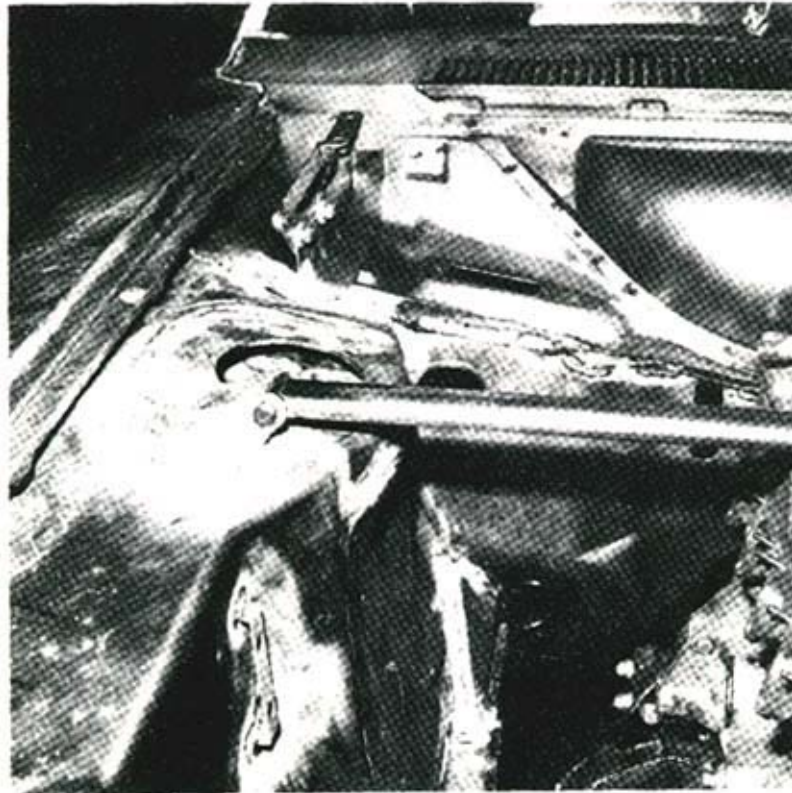
Strut brace fitted to works shell. Note simplicity, with mounting bracket in front of strut mount.
