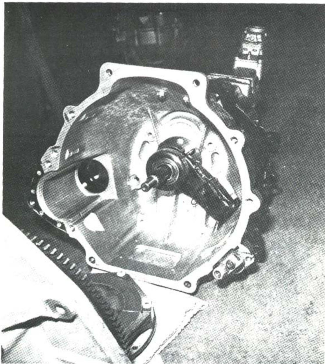
Inside the quick release bell housing, showing release mechanism with built-in trumpet.
